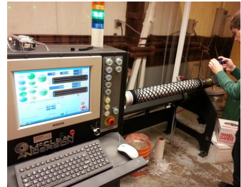
Figure 8.1. The Little Hornet filament winder is shown with one layer of yarn partially laid up.
